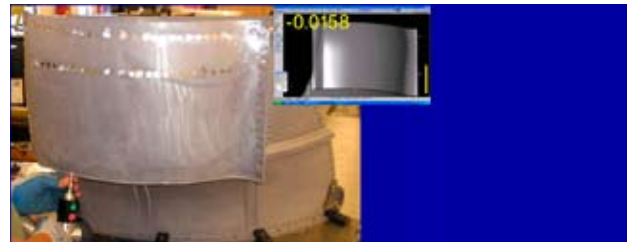
Creating a trim line for the mating cowlings from the CAD solid model using the FaroArm
