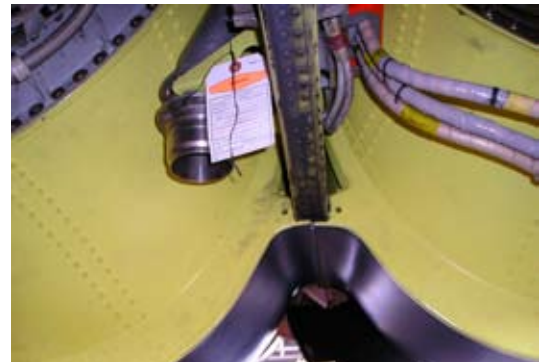
This photo shows the "after" condition of the bypass ducts built with the FaroArm system, and how their profiles and attach points now line up correctly.
