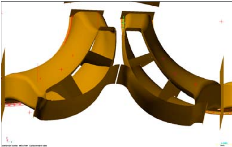
This photo shows the "after" condition of the bypass ducts built with the FaroArm system, and how their profiles and attach points now line up correctly.
